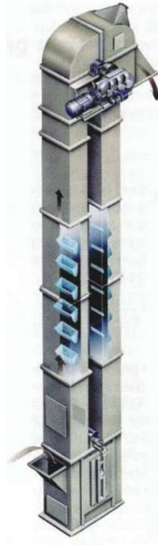
Figure D.20 – Bucket elevator
