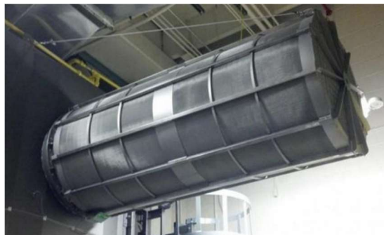
Figure 2 - Dust collector with flameless skimming device
