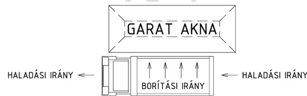
Figure D.6 - Reception room with a sinkhole, without masonry
