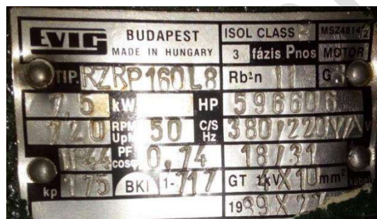
Figure 2: Data plate on a motor with explosion proof design installed before the ATEX directive entered into force
